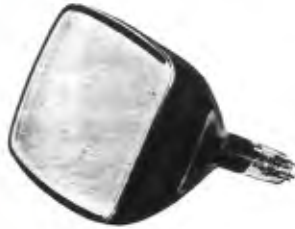
Fig.3: the 5-inch 140CB4 CRT was designed for this application. It provides excellent contrast.
