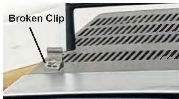
Fig.11 (above): pretty much all Sony 5-303E sets will suffer from a broken plastic antenna clip by now, as the plastic becomes brittle over time.
