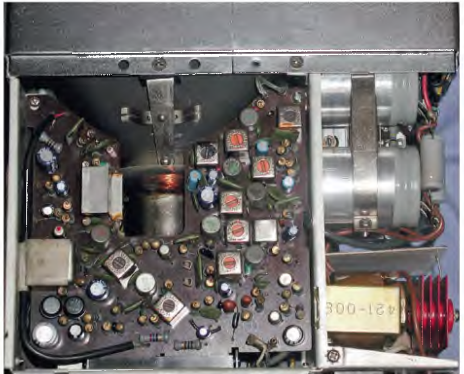
Figs.8(a) & (b): the signal board carries the remaining TV circuitry not on the upper "deflection" board.
