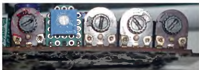
Fig.17: one of the preset pots had gone bad, and since I couldn't easily source a replacement, I rigged up a modern trimpot of the same value to fit in the same location.
