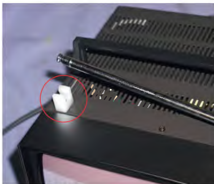
Fig.11 (above): pretty much all Sony 5-303E sets will suffer from a broken plastic antenna clip by now, as the plastic becomes brittle over time.
