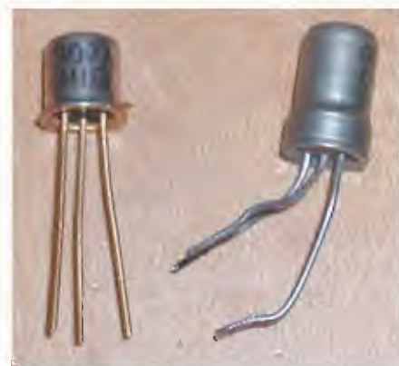
Fig.18: despite being a silicon transistor, the BC107A (left) was a perfectly fine replacement for the internally faulty germanium 2SD65 (right) in my set. That's only because of the way it was used in the circuit though; it isn't operated in a linear manner. If it were, a germanium replacement with similar properties would have been required.
