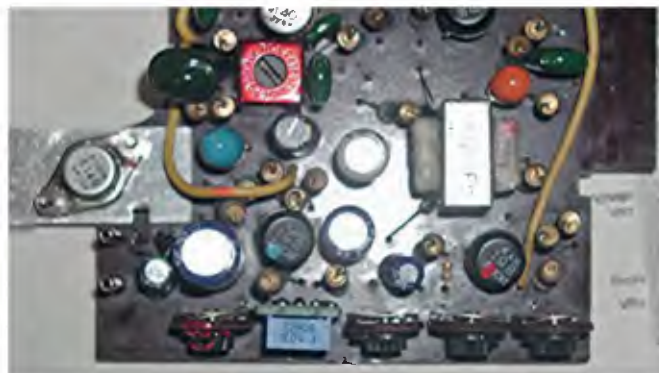
Fig.17: one of the preset pots had gone bad, and since I couldn't easily source a replacement, I rigged up a modern trimpot of the same value to fit in the same location.
