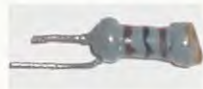
Fig.19: this innocent-looking 100 \Omega 5% resistor was the source of all my frustrations! It measured OK by itself, but when current passed through it, its resistance varied wildly.
