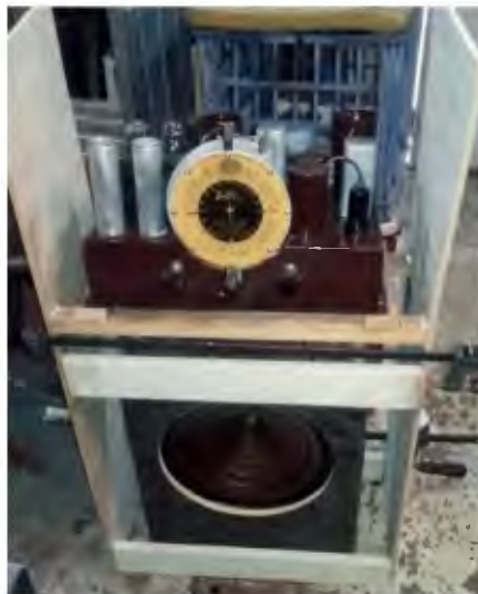
Fig.26: I mounted the chassis just high enough so that the speaker board would fit below it. This turned out to be a mistake – I could easily have mounted it higher, but I didn't think of it at the time! By the time I realised this, it was too late...
