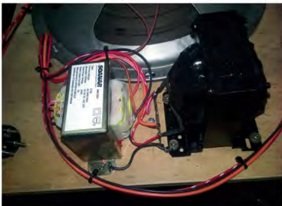
Fig.20: the rear of the speaker showing how I mounted the output transformer I made by modifying a mains transformer, plus the filter choke and series resistor for the HT supply (replacing the field coil of the original electrodynamic speaker).
