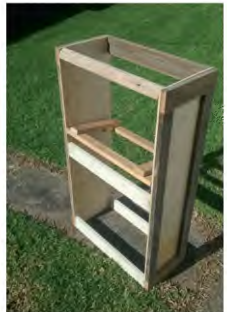
Fig.27: I added bracing to the frame so it would not fall apart if moved with the chassis inside.
