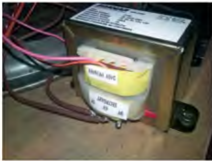
Fig.22: the modified transformer after reassembly. Note the red tape providing the 'air gap' in the core to prevent saturation from the unavoidable direct current flow.
