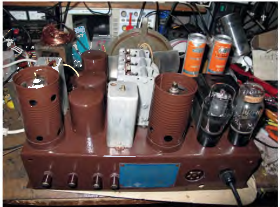
Fig.17: ahh, much better. The top of the chassis after restoration. The soup can shields are a 'love it or hate it' affair. I happen to think they look pretty decent.
