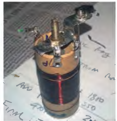
Fig.15: the oscillator coil after I'd finished making my modifications to suit the set under construction.
