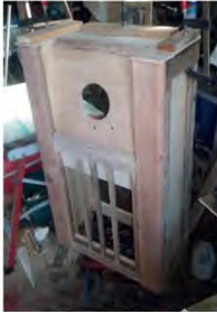
Fig.28: I added some profiled pieces of timber at the top to resolve the shape. You can also clearly see the frame I made from the speaker grille in this shot.
