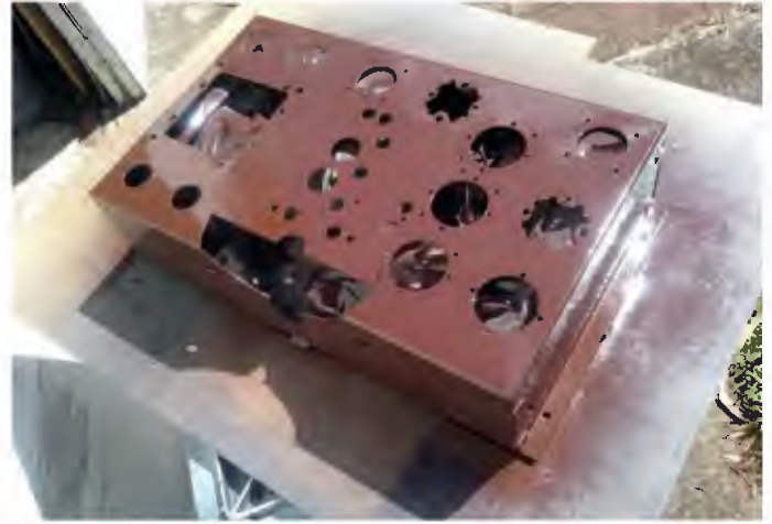
Fig.4: with the worst of the rust gone and a coat of primer plus a thick coat of paint, it's now ready to rebuild.
