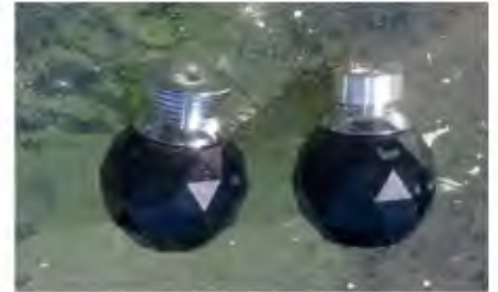
Fig.29: the original Bunnings (left) and modified (right) knobs. The modified knobs were made using a lathe to better suit a 1950s style.
