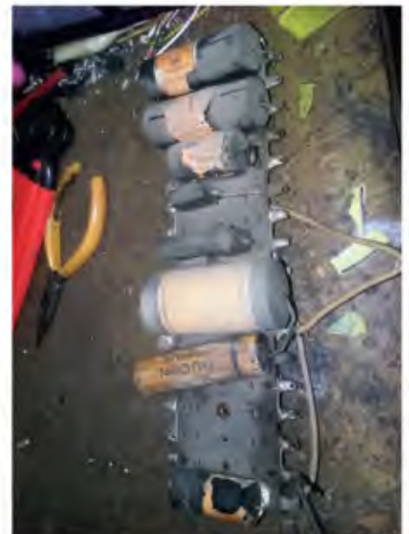
Fig.6: some of the larger capacitors were hiding under the central tag strip.
