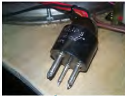
Fig.23: the Bakelite speaker plug I fabricated from a discarded valve base and a scrap dome.
