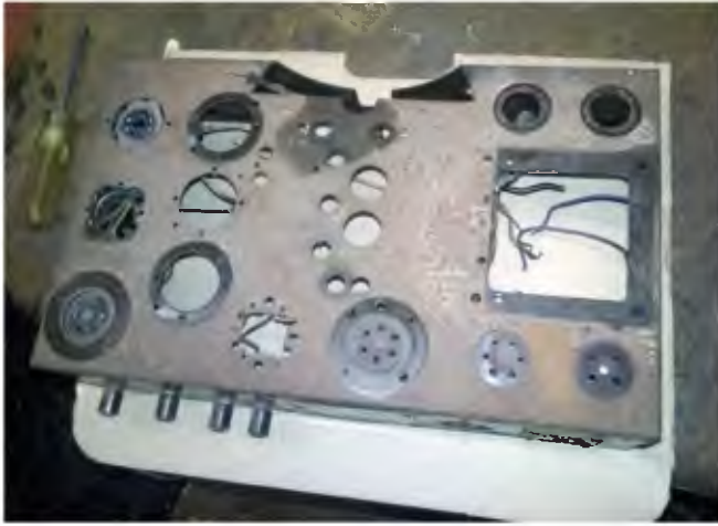
Fig.3: the chassis after removing all the parts but before rust treatment.
