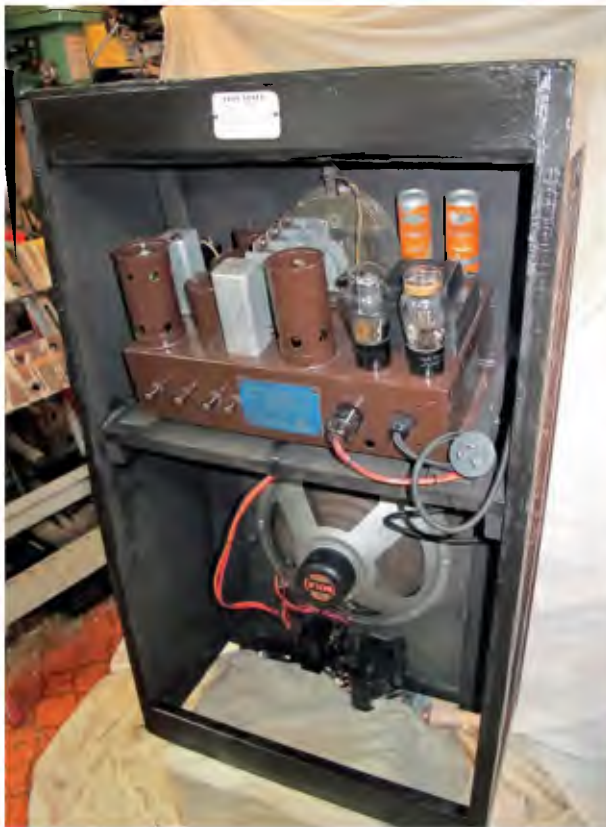
Fig.32: the rear view of the completed 'rat radio'. I'm pleased with how tidy it is.
