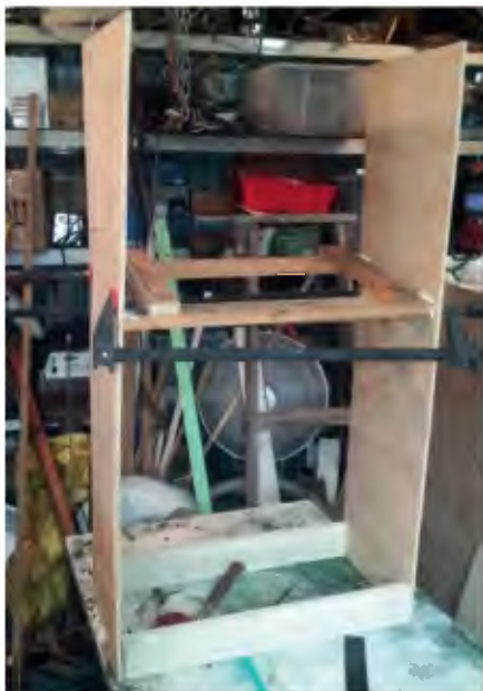
Fig.25: you can see how the chassis cradle sits at an angle so that the dial appears straight-on when you look down at it.
