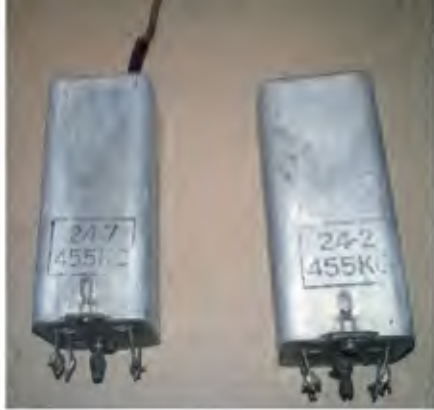
Fig.9: the two matched 1950s era intermediate frequency transformers I found in my collection that turned out to work pretty well.
