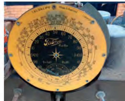
Fig.2: the dial didn't look too bad (besides the discolouration from the lamp's heat at the top), but it was pretty brittle. I added a protective layer to preserve it.
