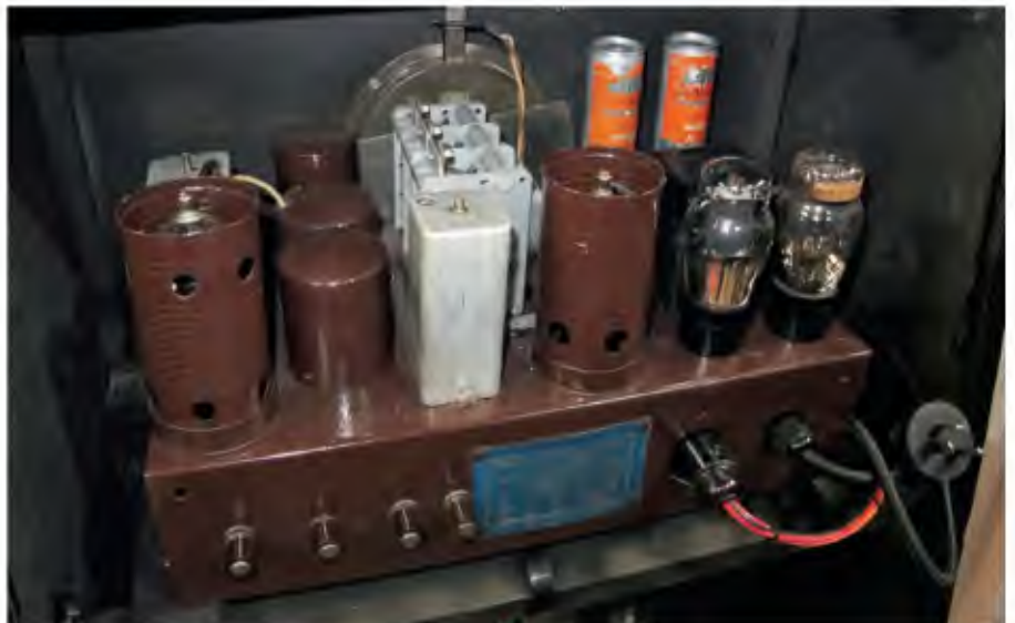
Fig.31: a close-up of the finished chassis mounted in the cabinet.
