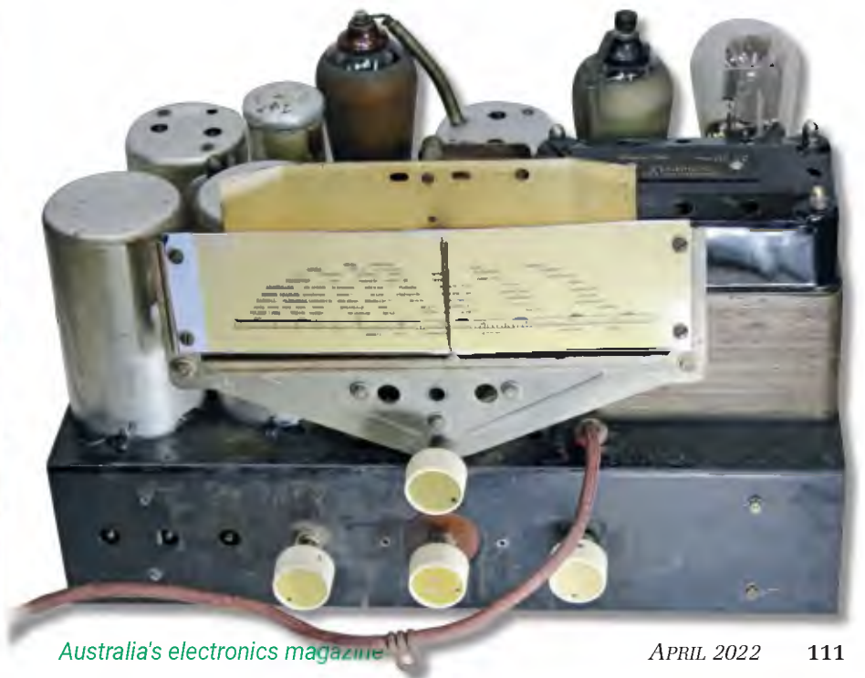
The restored tombstone radio, along with some shots of the chassis during restoration. Note that the photo below has the dial already repaired.
