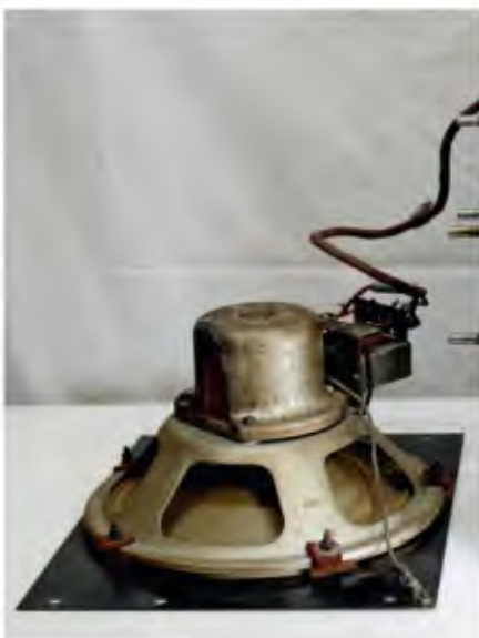
This speaker was not original, it was instead an Australian-made 8-inch Rola speaker of the same vintage.
