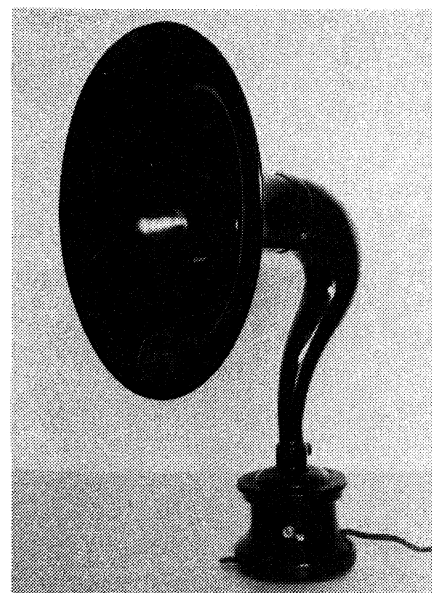
A British 'Claritone'; adjustment is by means of the lever projecting from the base.
