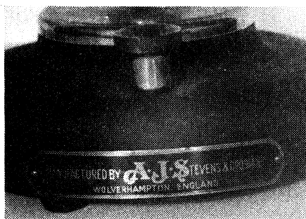
Not a piece of a vintage motor cycle, despite the name plate! The knurled knob is the diaphragm spacing control.
