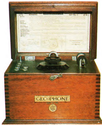
Fig.3: The British GEC variometer tuned Gecophone crystal set No1 of 1922, in a dovetailed mahogany case. Many sets of this era were similar in appearance to scientific instruments.
