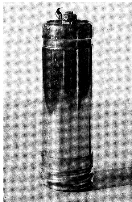
Fig.4: An interesting link in the evolution of the traditional wet electrolytic capacitor, this copper cased example was hidden inside the box alongside the power transformer. Note the threaded socket for easy changing in the event of failure.
