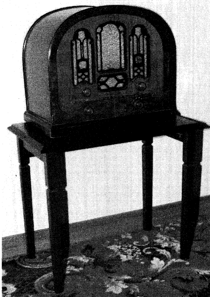
Fig.5: The eight-valve 708 of 1933 is a remarkable set for its size. A very early all wave receiver, coverage is continuous from 550kHz to 20MHz, with the RF stage used on all bands, and there are two 472.5kHz IF stages.
