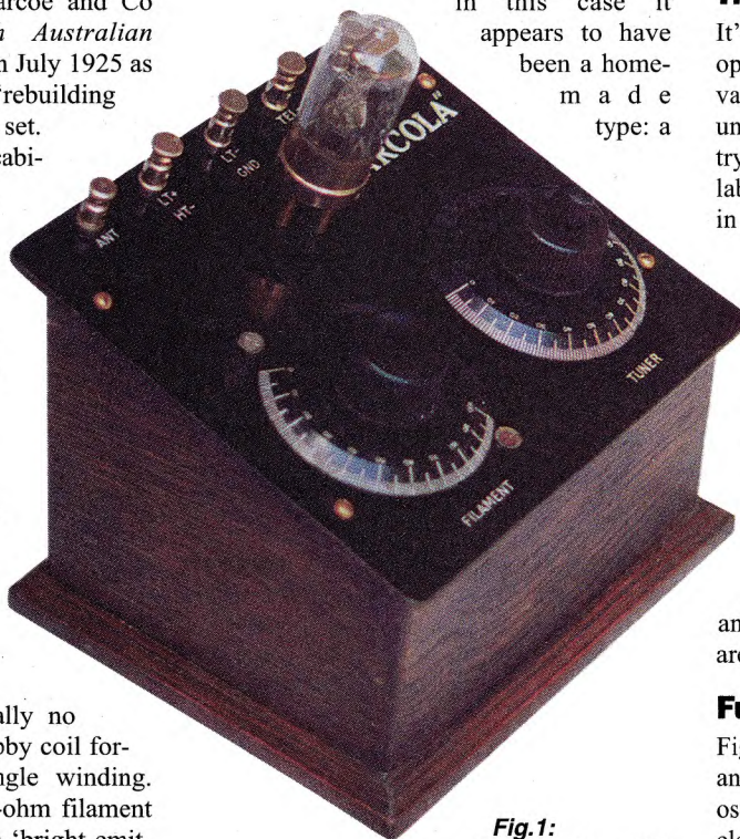
Fig.1: The little 'Varcola' set, which is really very simple and compact. It probably started life as a crystal set.
