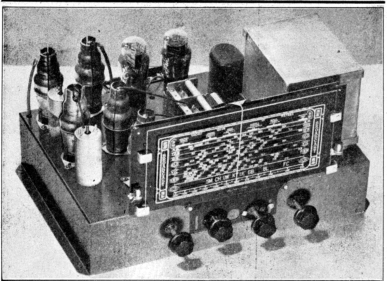
This picture gives a good general idea of the layout. It is very similar to that of an A.C. set except that the vibrator unit takes the place of the power transformer and rectifier. The speaker transformer can be seen at the rear of the chassis.
